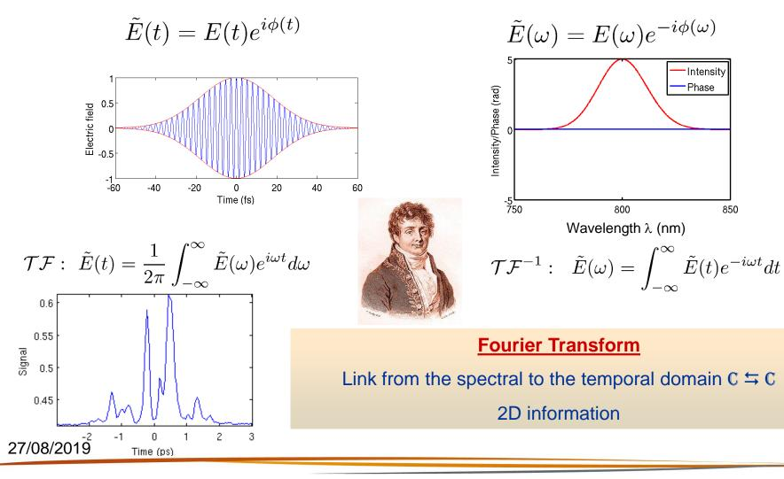
!! Representaiton !!It is always represented<br/>the spectral phase : $\phi(\omega)=\arg(E(\omega))$ And the spectral intensity $I(\omega) = |E(\omega)|^2$
